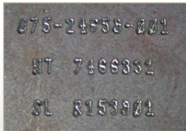
Typical punch marking for characters
